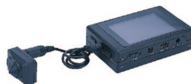
Connected /w the PVR via the attached Cable
